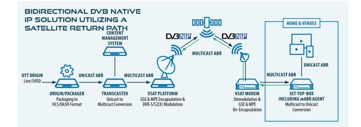
VOD (Video on Demand) and PDFs can be pushed out to receivers. Both live or linear distribution can happen unidirectionally or bi-directionally, where the bi-directional delivery utilizes a satellite return path using a VSAT platform.
