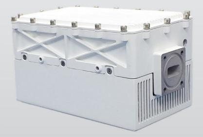
Lite 12W/16W Ku Band Block-Up Converter
