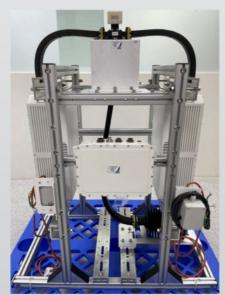
Compact 500W Phase-Combined C Band Block-Up Converter
