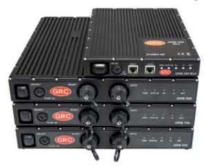
The GRM family of rugged iDirect Modems, including the GRM 950, 700, 200 and 200 Mini.
