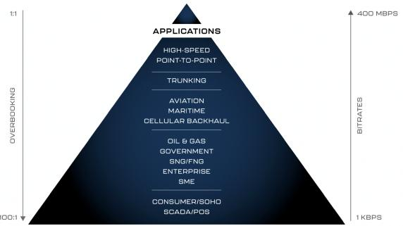
is typically found in SCADA, PoS and consumer or SOHO broadband. all the way to the higher fixed bit rate applications needed for cellular backhaul and maritime applications. Between the two, are applications requiring higher bandwidth and less sharing than the very bursty applications at the bottom of the applications pyramid, Satellite News Gathering (SNG), Government, Enterprise and Small- and Mediumsized Enterpises (SME), for example. Mx-DMA MRC will seamlessly handle all of these.
