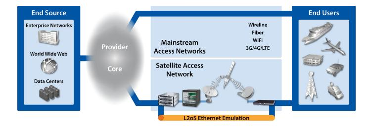
The platform's Protocol Processors and remotes serve as Ethernet switches that maintain MAC tables to make forwarding decisions based entirely on the information in the Ethernet header, passing entire Ethernet frames over the air. As a result, the platform behaves not unlike a simple Ethernet cable from the port entering the hub Protocol Processor to the port exiting the site remote.
