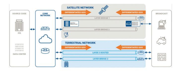
On top of having a wide range of IP-supported media available, an intelligent connection management system handles bandwidth fluctuations over each media, taking into account the different QoS these services require per terminal. In addition, the management system can also flexibly address the re-distribution of available satellite bandwidth over remote terminals that are communicating concurrently.
