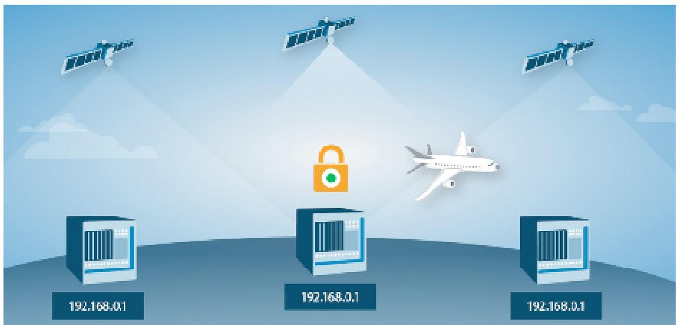
On an ST Engineering iDirect network, an aircraft can travel seamlessly across multiple satellite beams. In Automatic Beam Switching, a persistent IP address and a global acquisition key enable secure global travel with minimal service interruptions.
