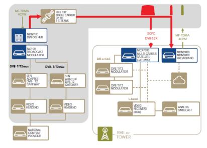
transmission is used in its most efficient way with DVB-S2X transmission, in combination with Equalink<sup>®</sup> 3. The set-up is optimal if a full transponder is filled up and used in saturated mode in which case Equalink<sup>®</sup> 3 is most efficient. DVB-S2X for enhanced efficiency over satellite results in more DTT multiplexes.
