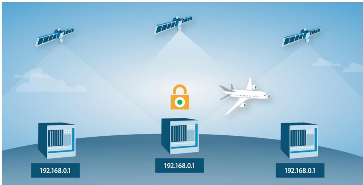
On an iDirect network, an aircraft can travel seamlessly across multiple satellite beams. In Automatic Beam Switching, a persistent IP address and a global acquisition key enable secure global travel with minimal service interruptions.
