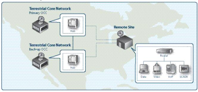
Organizations can link a primary and secondary hub to ensure complete network and system redundancy.
