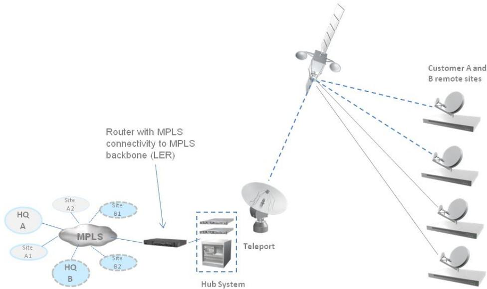
Figure 1: Integrate Customer Sites to MPLS Backbone
