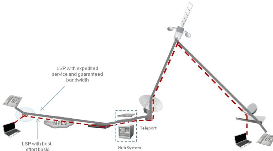
Figure 2: iDirect QoS to MPLS LSP Mapping
