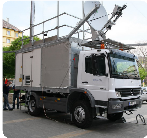
Pro-M's satellite-enabled mobile base station vehicle stands ready to provide TETRA communications.
